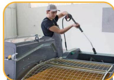
The hydro-cleaner available on request can operate directly from the hydraulic circuit. This choice allows completely independent **high speed washing** of your S28 R.
