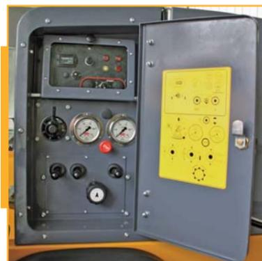
The control panel allows control of all functions by showing the state of operation. The control box is protected by a high resistance plexiglass door.
