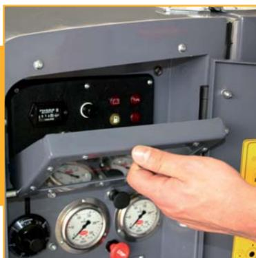
The hood is completely soundproofed. In addition, it is characterized by a very large opening.
