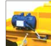
The vibrator ensures a quick and efficient screening
