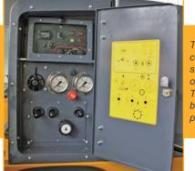
The control panel allows control of all functions by showing the state of
