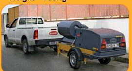
The new ALKO axle of 1000 kg with tires 165 guarantees an exceptional stability for safe towing even with normal motor vehicles. (Max 130 Km/h)
