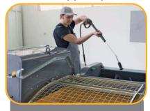
The hydro-cleaner available on request can operate directly from the hydraulic circuit. This choice allows completely independent high speed washing of
