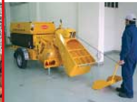
The scraping device facilitates loading the tank
