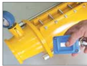
The CLB18 is equipped with a remote control with electric wire to start and stop pumping. A wireless remote control is available on demand.
